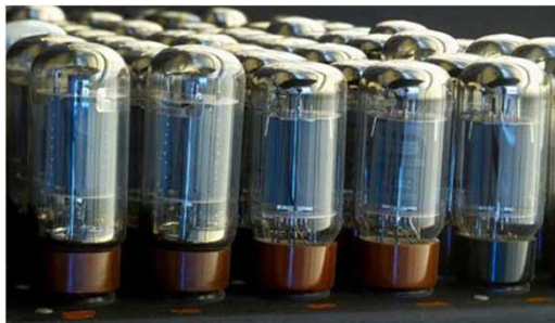
Vacuum tubes from the ENIAC computer
